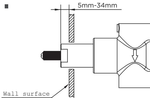
While placing the valve into wall, make sure that the adaptor protruding out from the wall surface is between 5~34mm as the figure indicates.
