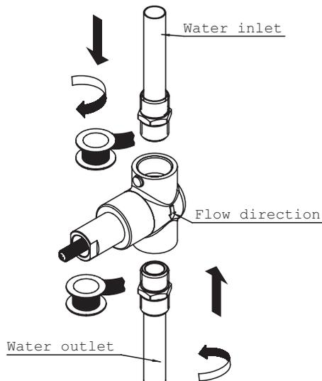
Connect the valve inlet and outlet with water pipes.
